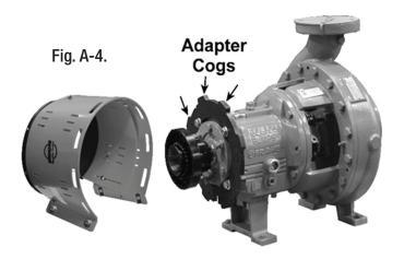
4. Ensure that all cogs and openings are seated securely, then close guard and tighten 3/8" captive fastener bolts securely as shown in Fig. A-5.
