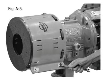
5. Extend the inner telescoping barrel (motor end) until it meets the surface of the motor. Ensure that there is no more than ¼" gap between guard and motor as shown in Fig. A-6. Tighten the hex head nut to hold extended telescoping portion in place.
