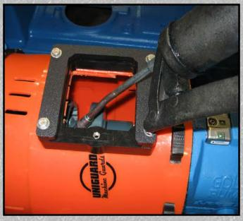
One of the many benefits of the **Inspection Window** is coupling lubrication access without guard removal.
