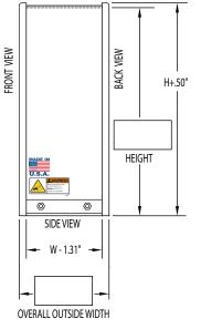
Height should equal = shaft centerline + 1/2 sheave dia. + 2.0" clearance
